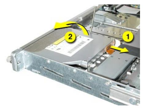
4. Remove the two screws that secure the side bracket to the original drive and remove the bracket from the drive. (Figure 4)
